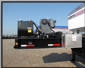
60 HP DEUTZ DIESEL POWER PACK
