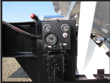
SEALED CONTROL PANEL W/ SAFETY SHUTDOWN SWITCH
